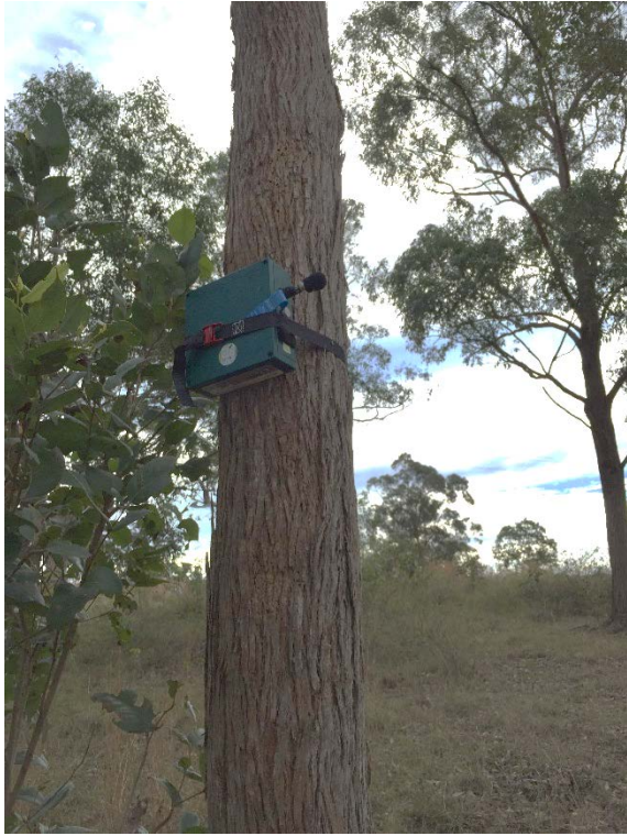
Song Meter set on site for acoustic recordings
