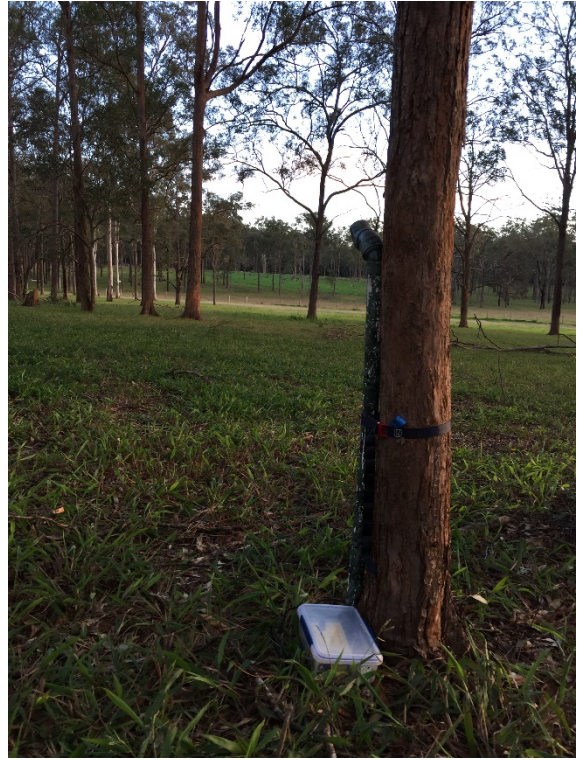
Anabat detector on site for ultrasonic recordings
